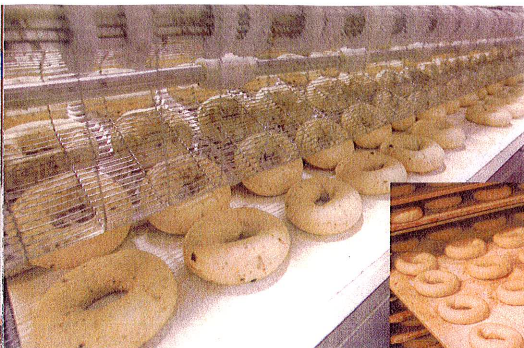
(Top) The wing loader system peels bagels off of boards and stages them for the boiling, seeding and baking process at 465 bagels-per-minute. (Right) Bagels are proofed for a minimum of 12 hours similar to those made in a traditional bagel shop.
