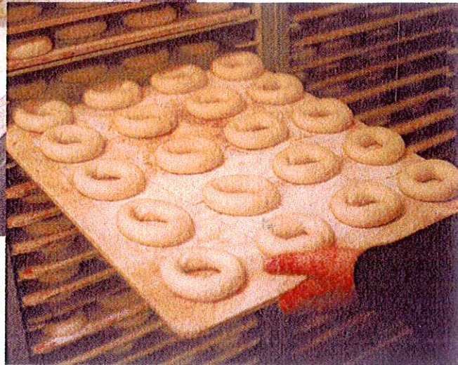
(Top) The wing loader system peels bagels off of boards and stages them for the boiling, seeding and baking process at 465 bagels-per-minute. (Right) Bagels are proofed for a minimum of 12 hours similar to those made in a traditional bagel shop.
